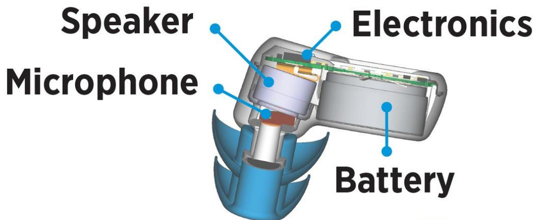
In full-size on-ear noise cancelling headphones the microphone element is located outside the ear. However, in QuietOn, the microphone that samples the sound is located right inside the ear canal! This means that QuietOn can more accurately produce anti-noise that results in good noise cancellation at the ear drum. By locating the microphone in the air volume of the ear canal, QuietOn is also able to reduce noise that is conducted by the skull into the ear.
