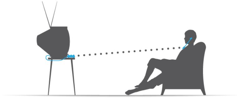
The transmitter is placed on a flat surface facing the seating area and is connected to the audio out port on the back of the television, satellite or cable box. The transmitter then sends audio wirelessly to the headset worn by the user. Volume and tone adjustments are available on the headset for creating perfect dialog clarity. TV Ears works separately from the TV volume (so the TV can be turned down or muted) and is compatible with any television.
