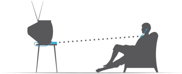
The transmitter is placed on a flat surface facing the seating area and is connected to the audio out port on the back of the television, satellite or cable box. The transmitter then sends audio wirelessly to the speaker system. Volume is controlled independently from the TV on the Speaker.
