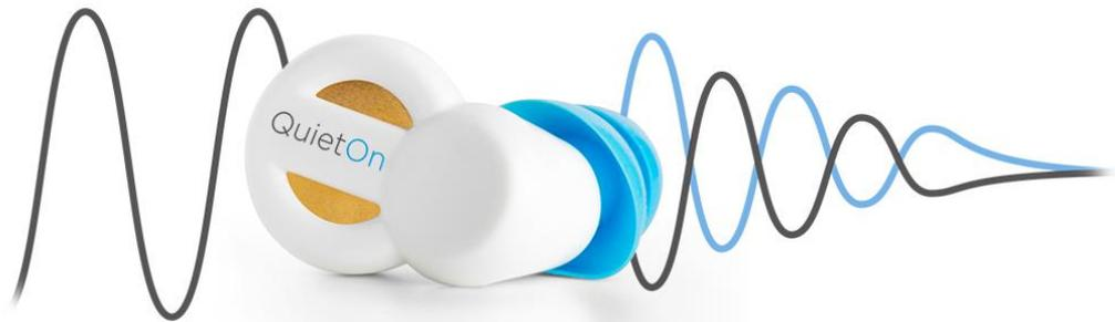
Active noise cancelling uses a microphone to sample the sound, and a speaker to create a phase-shifted sound that cancels the original sound.
