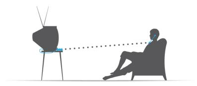
The transmitter is placed on a flat surface facing the seating area and is connected to the audio out port on the back of the television, satellite or cable box. The transmitter then sends audio wirelessly to the headset worn by the user. Volume and tone adjustments are available on the headset for creating perfect dialog clarity. TV Ears works separately from the TV volume (so the TV can be turned down or muted) and is compatible with any television.
