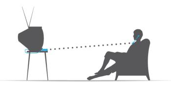
The transmitter is placed on a flat surface facing the seating area and is connected to the audio out port on the back of the television, satellite or cable box. The transmitter then sends audio wirelessly to the speaker system. Volume is controlled independently from the TV on the Speaker.
